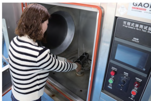
成品防水检测 To detect waterproof performance of end product.
