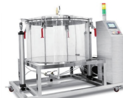
成品气密性测试 To do Air tightness test of end product.
