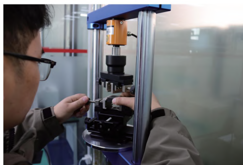
成品强度、拉力检测 To detect intensity strength and pull of end product.
