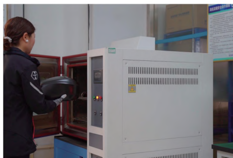
成品高低温检测 To detect extremely cold and high temperature of end product.
